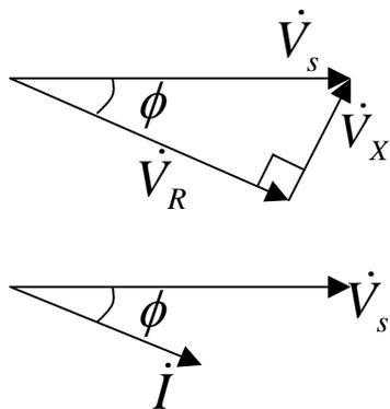
$$\begin{aligned} \dot{I} &= \frac{\dot{V}_s}{R + jX} = \frac{V_s \varepsilon^{j\theta}}{\sqrt{R^2 + X^2} \varepsilon^{j\phi}}, \theta = 0 \text{ とする。} \\ &= \frac{V_s \varepsilon^{-j\phi}}{\sqrt{R^2 + X^2}}, \tan \phi = \frac{X}{R} \end{aligned}$$
